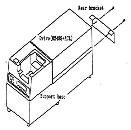
Figure 1-3. Drive with ACL (5-cartridge) Desktop Configuration
